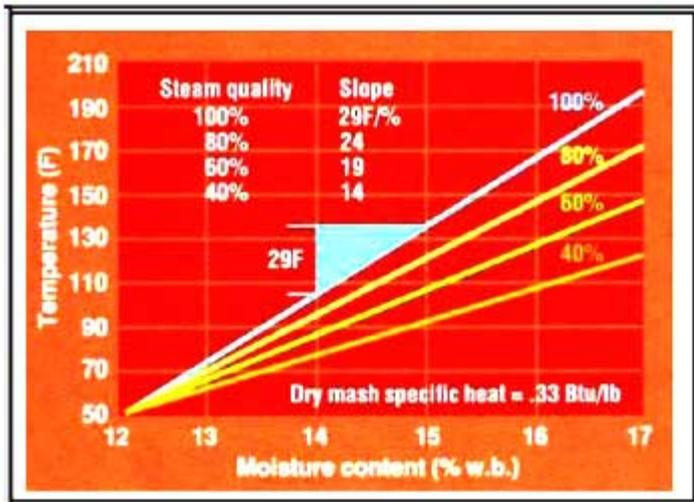
Figure 4 illustrates the rise in temperature per moisture percent.
